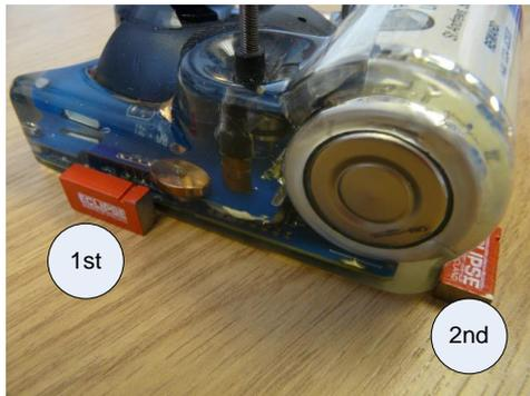
**Note:** The order in which the two magnets is positioned against the tag is important for programming. The magnet on the side of the tag **must** be positioned first, **then** the magnet to the rear of the tag.
