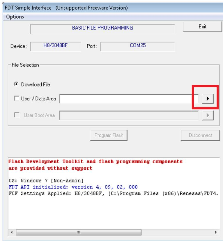
Navigate to the “.mot” file to load on to the tag
