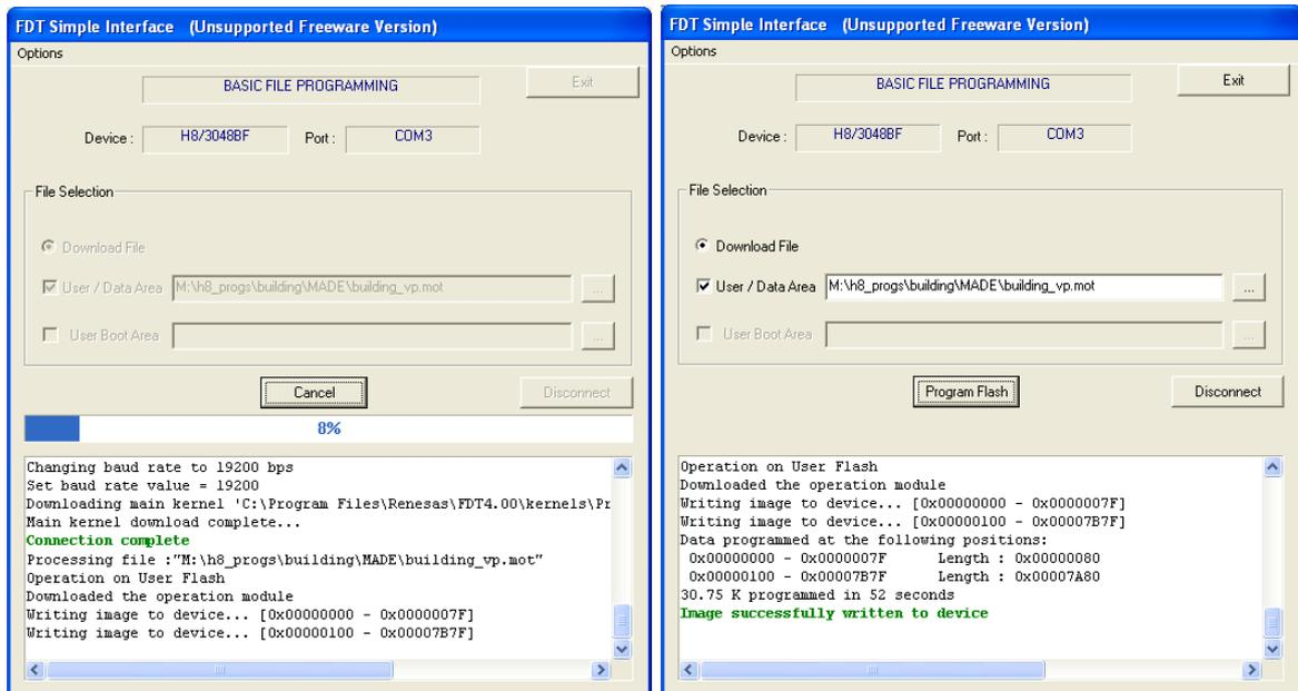
When programming has completed successfully, click “Disconnect” and remove the magnets from the tag. The tag should restart and indicate that it is in standby mode by a double flash of the red LED near the antenna.
