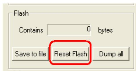
necessary to click “Reset Flash” before the first run to prepare the tag to log data. The reported size of the flash contents should return to zero.
