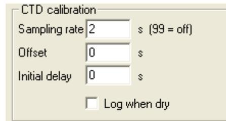
The “Initial delay” field specifies a pause, in seconds, before sampling begins. This is to avoid wasteful sampling if a long stabilisation period is required. The maximum permitted value is 65,500 (about 18 hours).
