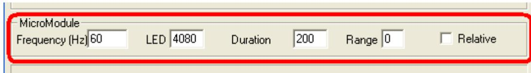
The fluorimeter pulses with a 1:1 duty cycle. The range of possible frequencies is 0.1 – 2000. Default 60
